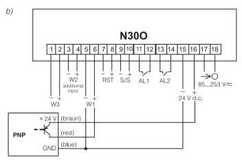
Fig. 5. Connection of the sensor with the OC Output:
