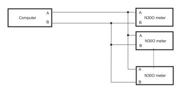
Fig. 13. Connection Way of the RS-485 Interface
