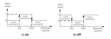
Fig. 12. Alarm types: a) n-on, b) n-off c) on d) off.
