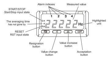
Fig. 7. Description of the Meter Frontal Plate
