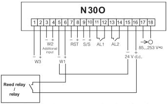
Fig. 6. Connection of the sensor with the Reed Relay/ Relay Output Type
